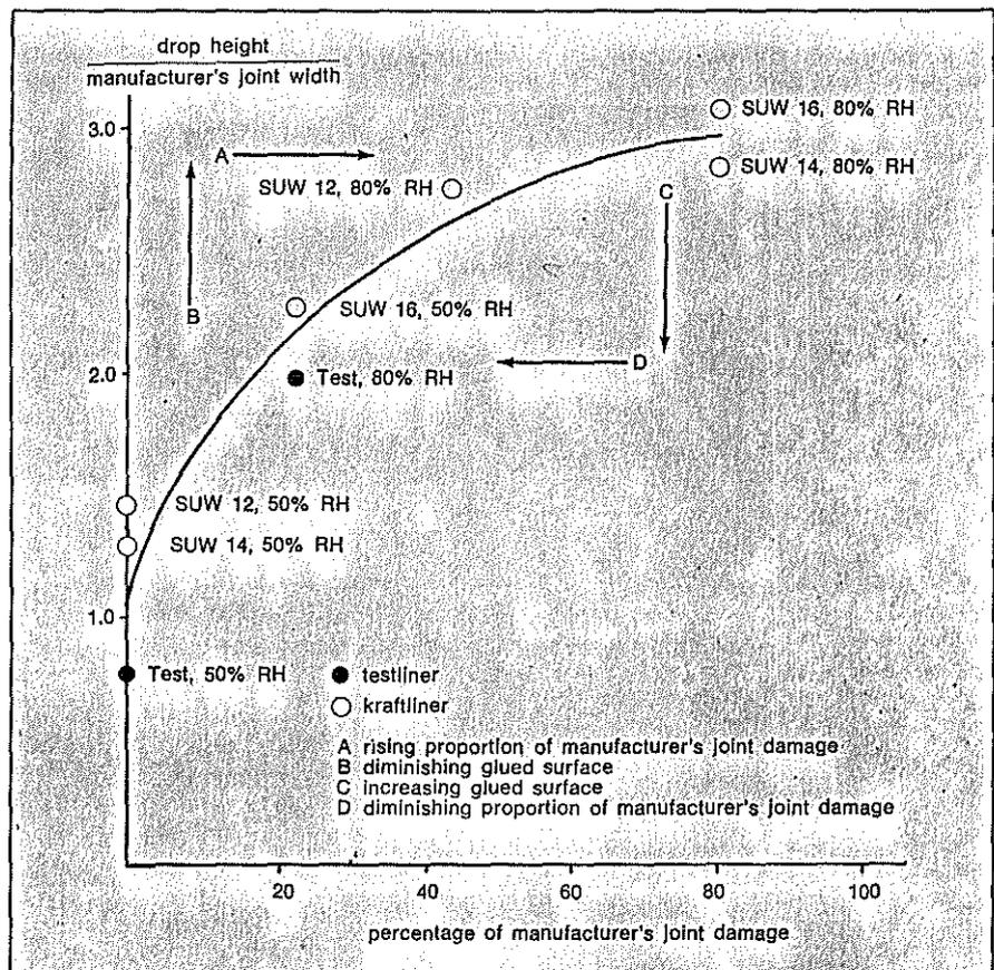
Figure 1. Relation between drop height + manufacturer's joint width and proportion of manufacturer's joint damage.
